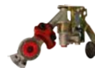
Swing-Away Gladhand Rotates A Full 180° For Easy Air Line Coupling.
