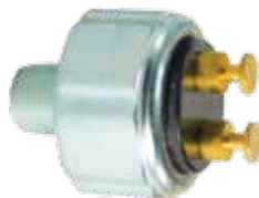
422709 STOP LAMP SWITCH NORMALLY OFF SPST OPERATES 60-120PSI CONTACT CLOSED AT RISING PRESSURE
