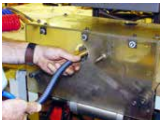
The final stage of creating a coiled tubing set is to attach the brass ends.
